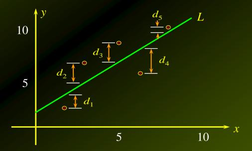
Suppose the regression line L is y = f(x) = mx + b, where m and b are to be determined.
