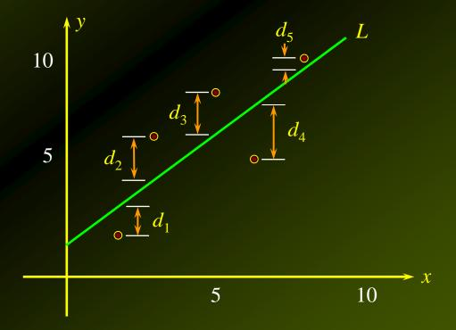
The principle of least squares states that the straight line L that fits the data points best is the one chosen by requiring that the sum of the squares of  $d_1$ ,  $d_2$ ,  $d_3$ ,  $d_4$ , and  $d_5$ , that is
